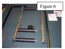
If the nuts do not come loose on one or both of the two rear drums, using a wrench on both ends of a drum, remove whichever nuts you can to separate the frame rails. This will be all the disassembly required to remove and replace both belts. Reverse the disassembly steps for re-assembly.
