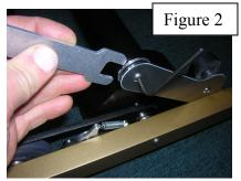
Release the tension on the flywheel belt by sliding the belt off the tensioner idler wheel. The belt will then be loose.
