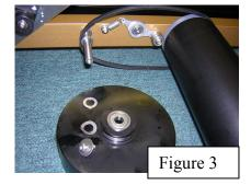
Remove the inboard bolt along with the flat washer, curved washer and thin washer. Please note the relative order of these 3 items for reassembly. The flywheel should then slide off the shaft. Lift the drive belt off the flywheel as you go.
